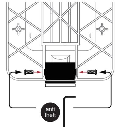
**4** Put the head tube dampener on the clamp. The 3 pins on the dampener fit into the holes on the clamps.
