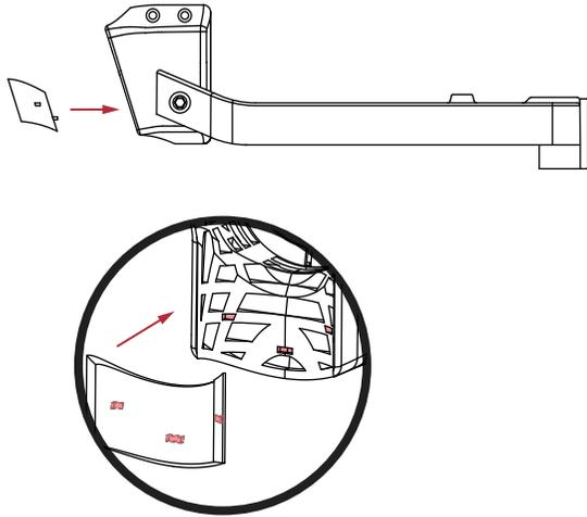
**5** Connect the light wires and install the assembled front carrier. Push the front carrier as close to the frame as possible so that the pins on the inside of the clamp inserted into the holes at the front of the top tube.
