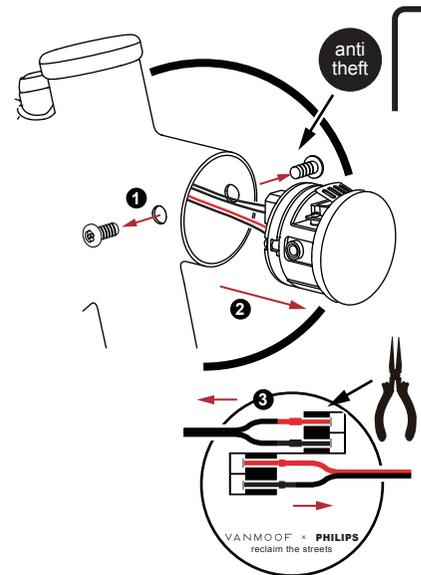
**2** Connect the wires coming from the carrier to the light. The connectors with two BLACK wires go to the "In & ~" connection. The connectors with RED-BLACK wires go "to rear".
